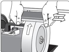
*Grade the stone by pressing the fine side onto the stone for 20–30 seconds. Use a high pressure.*
