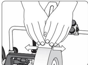
*Grind the tool as usual. The picture shows a plane iron in the SE-77 Square Edge Jig.*
