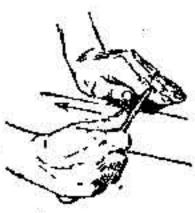
Turn the edge with a few firm strokes of the Burnisher on the bevel side of the blade. The scraper can be held in any of the three ways shown above.
